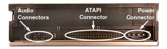
Power Connector Power is supplied to your DVD-ROM drive by the connection with your computer's +5V/+12V power cable to the power socket at the back of drive. One side of the plug has chamfered edges, so the power connector fits only one way
